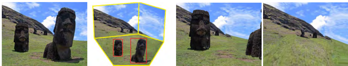
Figure 14: Example of 3D walkthrough. Left to right: the input image, the 3D model, and the novel views.
