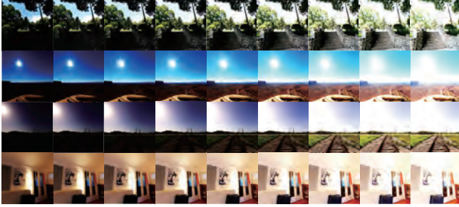
Fig. 4. Examples of bracketed images created from the HDR datasets. Exposures are selected to avoid completely white or black regions.
