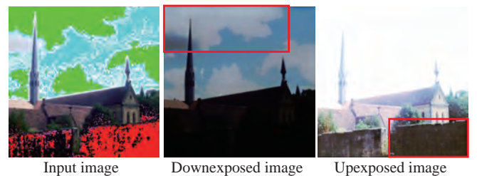
Fig. 9. Artifacts of repeated patterns caused by using adversarial loss. From left to right, the input LDR image; the downexposed LDR image, and the up-exposed LDR image.
